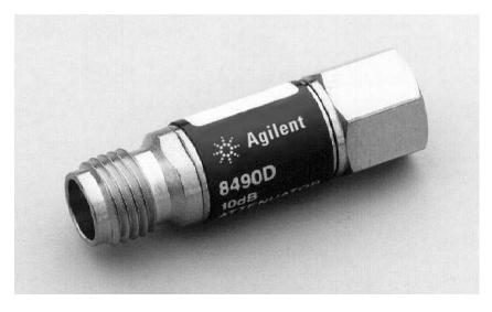
The Agilent Technologies 8490D family is a line of precision fixed coaxial attenuators with performance specified up to 50 GHz. These attenuators use the 2.4 mm coaxial connector, which exhibits excellent performance from dc to 50 GHz. The 8490D family has attenuation values of 3, 6, 10, 20, 30, and 40 dB.
